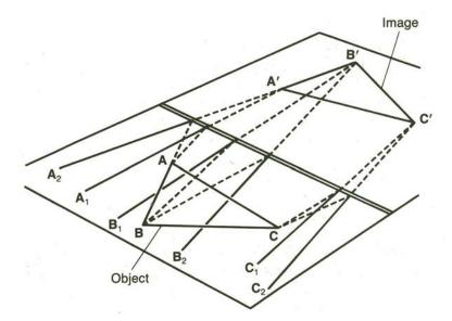
Figure 3: Finding the images of three pins.
